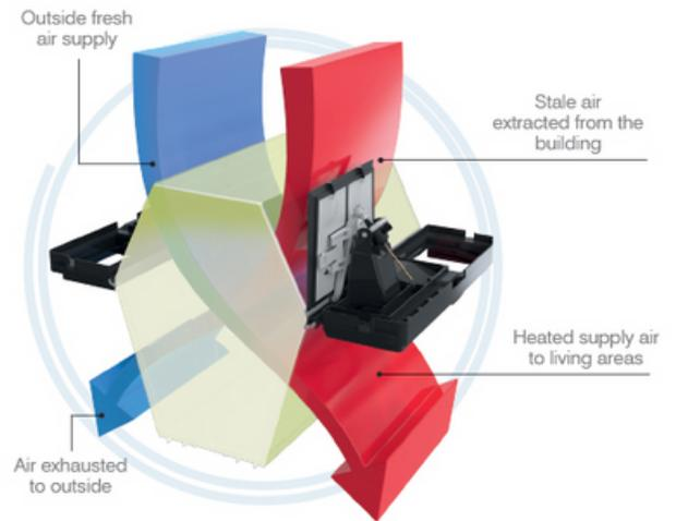
Enveloped can also supply and install decentralised ventilation, eliminating the need for ducting. This is ideal for small units and apartments where space is a premium, while still maintaining heat-recovery benefits.
